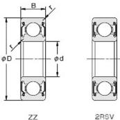
Allowable Allowable D В r(min) d radial load rotation Bearing No. Ν min<sup>-1</sup> mm mm mm mm SS 6800 10 19 5 0.3 170 2000 SS 6900 10 22 6 0.3 215 2000 SS 6000 10 26 8 0.3 370 2000 SS 6200 10 30 9 0.6 410 2000 SS 6300 35 2000 10 11 0.6 650 SS 6801 12 21 5 0.3 155 2000 SS 6901 12 24 6 0.3 230 2000 SS 6001 12 28 8 0.3 410 2000 12 32 SS 6201 0.6 545 2000 10 SS 6301 12 37 12 1.0 775 2000
